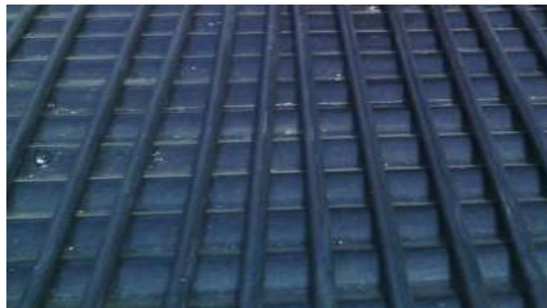
Figure 3 Attached fluid pipe onto the absorber plate
