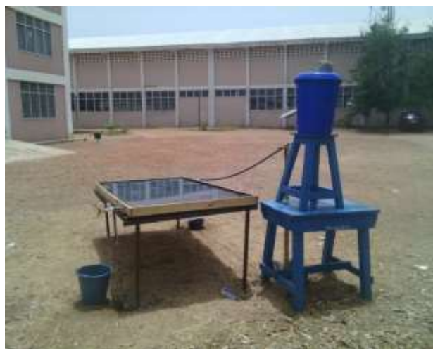
Figure 4 The prototype of solar water heater for the HCIM Department of Bolgatanga Polytechnic
